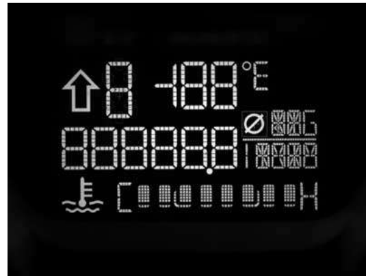
Figure 3: A monochrome camera captures an image of the entire LCD display. On the systems host PC, a set of calliper tools are run in sequence over each segment in the display images to look for edge transitions in the image from dark to light. In doing so, the software determines whether or not each segment of the display has been illuminated.
